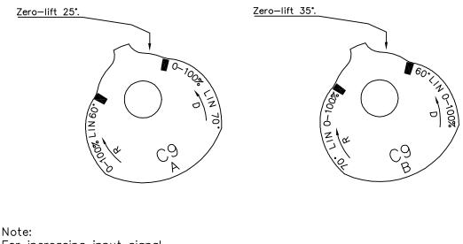
For increasing input signal, "D" stands for Direct(CCW) rotation and "R" for Reverse(CW) rotation.
