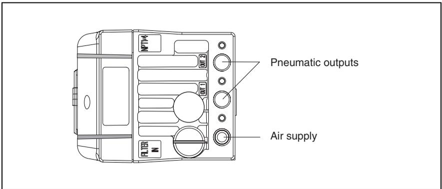
**Fig. 15 Pneumatic connections**
