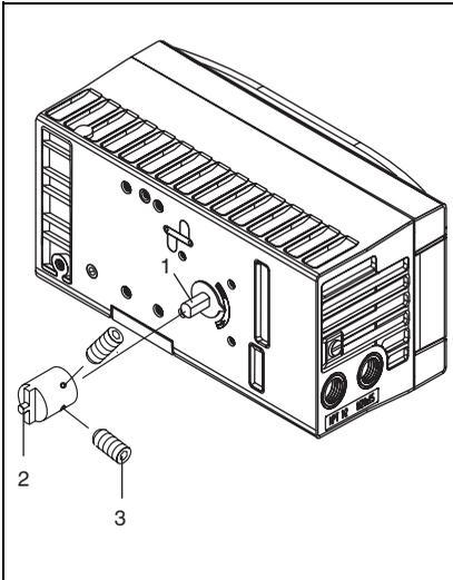
Fig. 12 Mounting the adapter
