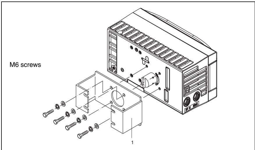
Fig. 13 Attaching the mounting bracket to the positioner
