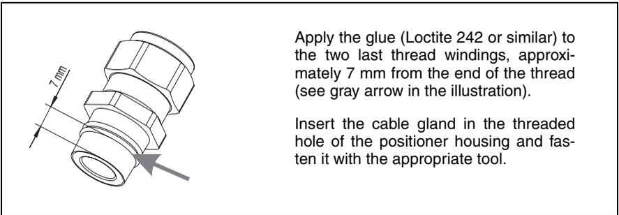
**Fig. 18 Fastening the cable gland 1/2 NPT**
