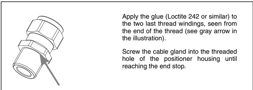
**Fig. 19 Fastening the cable gland M20 x 1.5**
