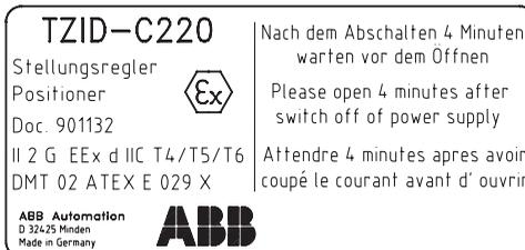
**Fig. 1** Type plate indicating the degree of explosion protection
