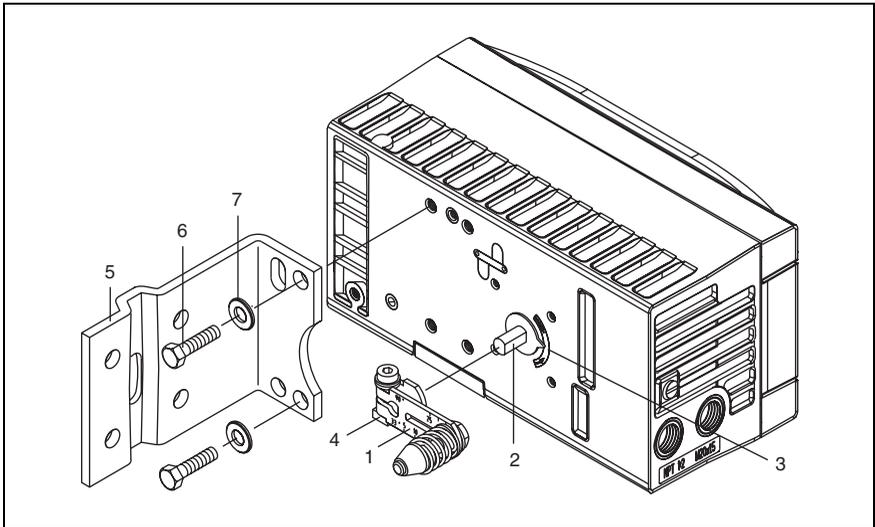
**Fig. 7** Mounting lever and angle bracket to TZIDC-220
