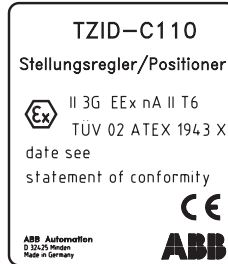
Fig. 1 Type plates indicating the degree of explosion protection
