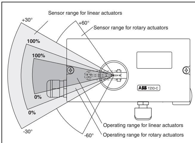
When mounting the positioner, ensure that the transfer of the stroke or rotation angle for the position feedback is correct. The maximum rotation angle is 60° for mounting to linear actuators and 120° for mounting to rotary actuators. The minimum angle is always 25°.
