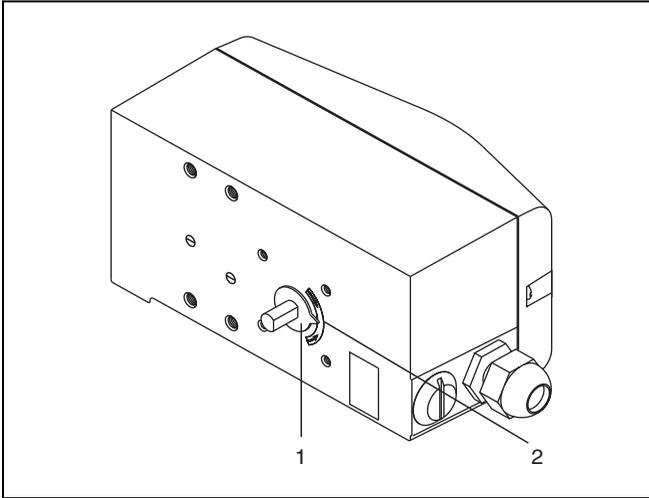
The arrow (1) on the feedback shaft (and thus the lever) must travel within the area marked with the small arrows (2).
