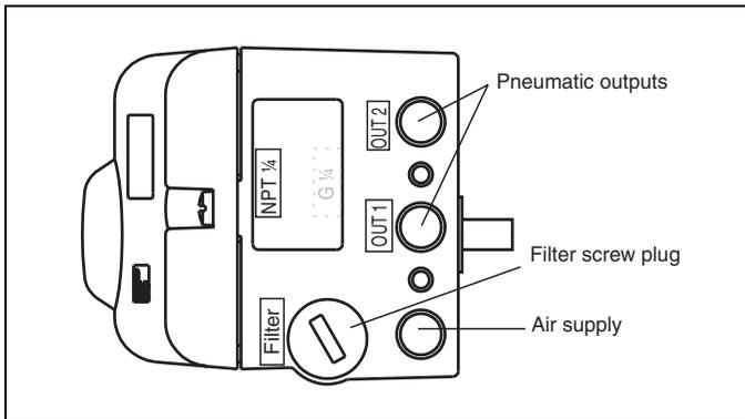
**Fig. 15 Pneumatic connections**
