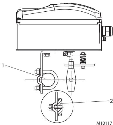
Fig. 2: Mounting to linear actuators to DIN/IEC 534
