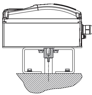
Fig. 3: Mounting to rotary actuators to VDI/VDE 3845
