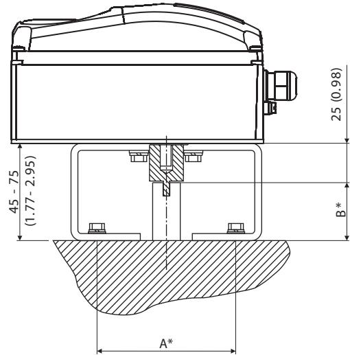
Fig. 19: Mounting to rotary actuators to VDI/VDE 3845
