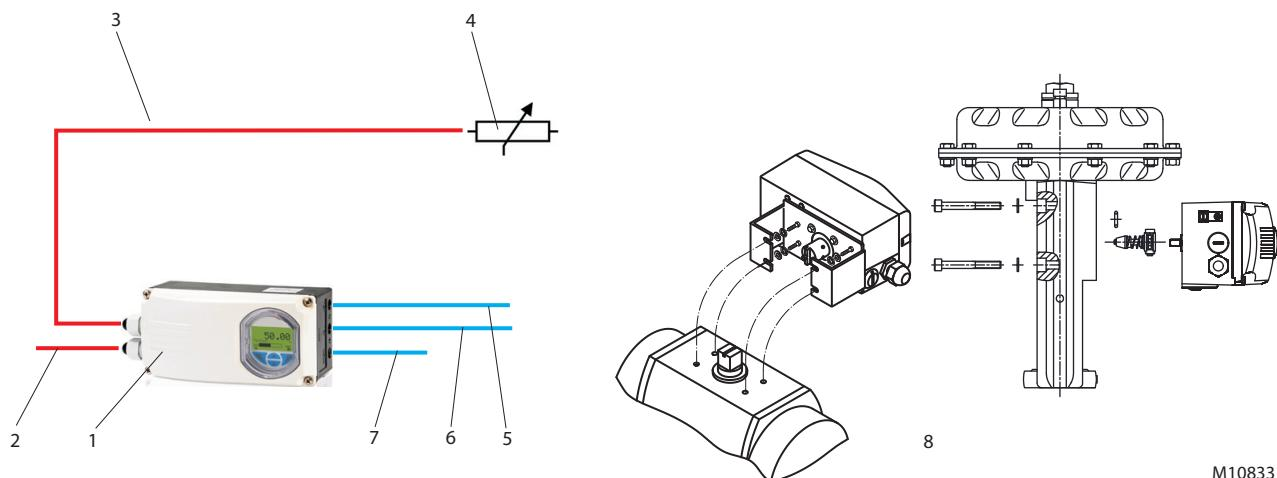
Fig. 28: D500 control unit for remote sensor
