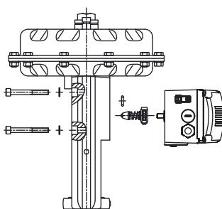
Fig. 4: Integral mounting to control valves
