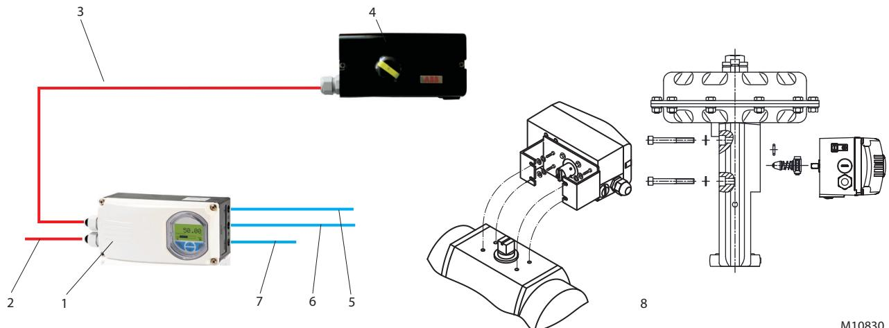
Fig. 25: D500 control unit with remote sensor
