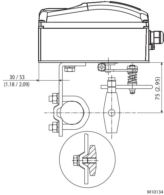
Fig. 18: Mounting to linear actuators to DIN/IEC 534
