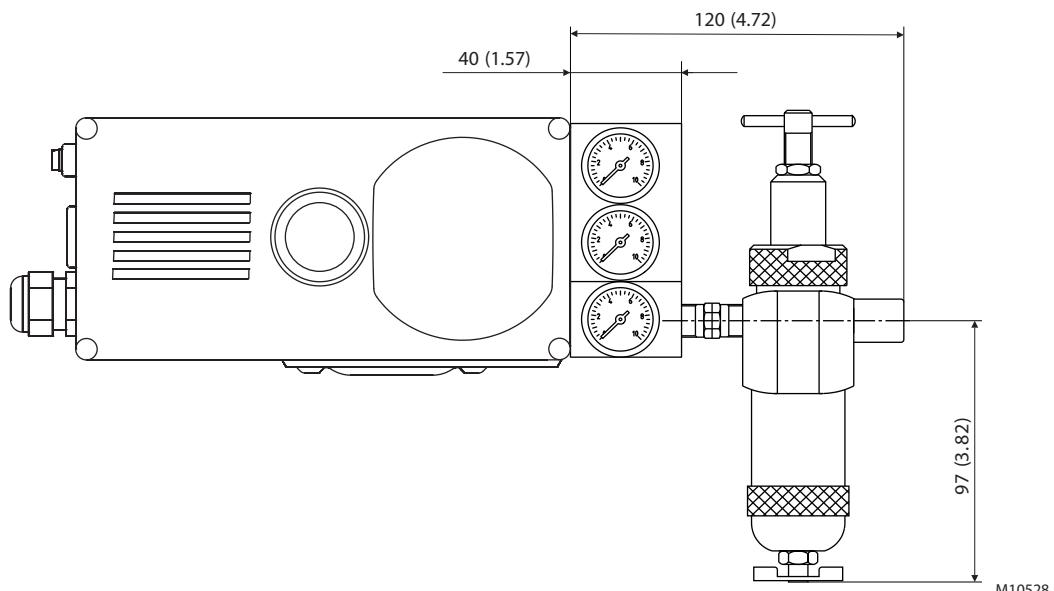
Fig. 15: D500 positioner with pressure gauge block and filter regulator mounted
