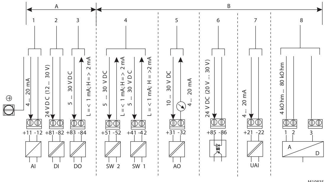
Fig. 30: Connection diagram of the D500 control unit
