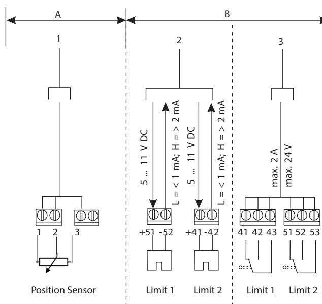
Fig. 31: Connection diagram to the D500 remote sensor
