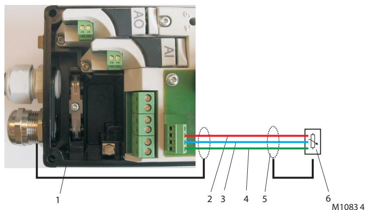
Fig. 29: Electrical connection
