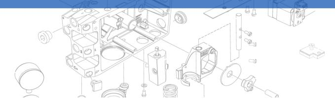
A positioner is an instrument connected to the stem of the valve/actuator. This makes the positioner unique because it is the only instrument with a direct connection to the process that can also change the process. A positioner is also beneficial because it directly responds to the process changes and forces that move the valve trim.
