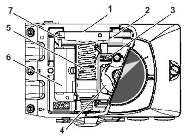
continue to hold the balance arm up and tighten the cam nut. Once the cam nut is tightened release the balance arm, the positioner is now set to operate from 4mA open to 20mA closed.
