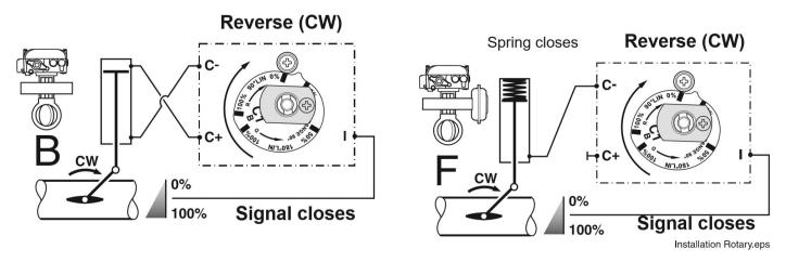
Here is a step by step procedure in getting from 4mA closed and 20mA open to 4mA open and 20mA closed.
