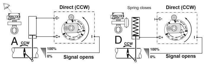
The customer would now like the opposite from their valve. They would like to have open at 4mA and closed at 20mA. The diagrams below are 4mA open and 20mA closed. The double acting is on the left and single acting is on the right.
