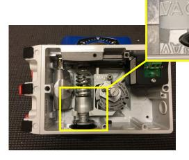
The above procedures will set the zero and span adjustments to the middle of their respective adjustment ranges and should be a good point to start calibration.
